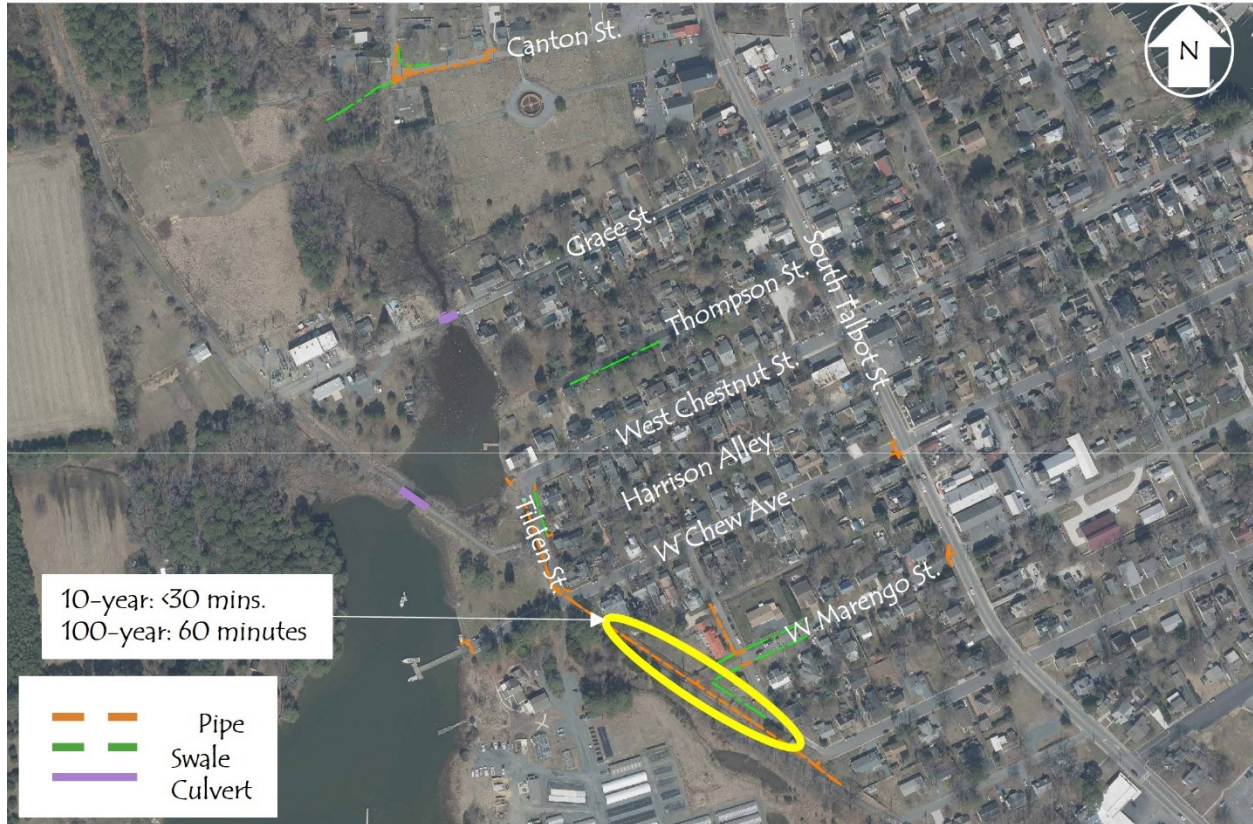
Figure 15 - 2050 Stormwater Flooding Duration at St. Michaels Nature Trail
