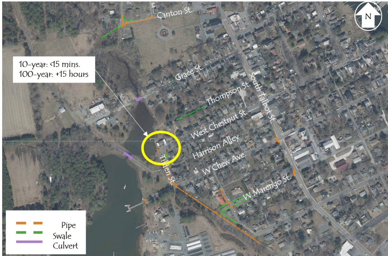
Figure 12 - 2050 Stormwater Flooding Duration at West Chestnut St. and Tilden St.
