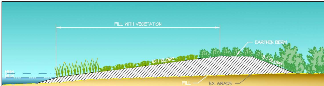
Figure 17 - Earthen Berm with Living Shoreline
