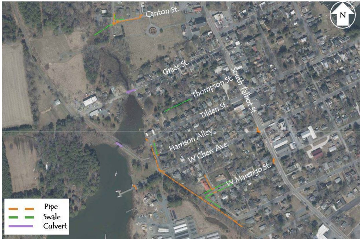
Figure 4 - Stormwater Management Features
