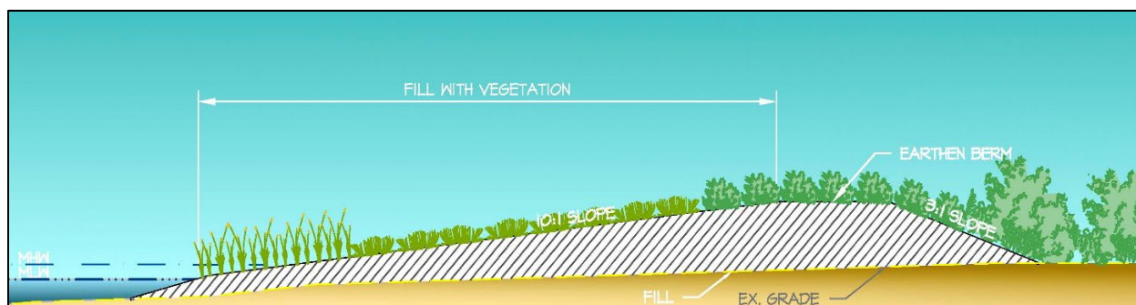
Figure 17 - Earthen Berm with Living Shoreline
