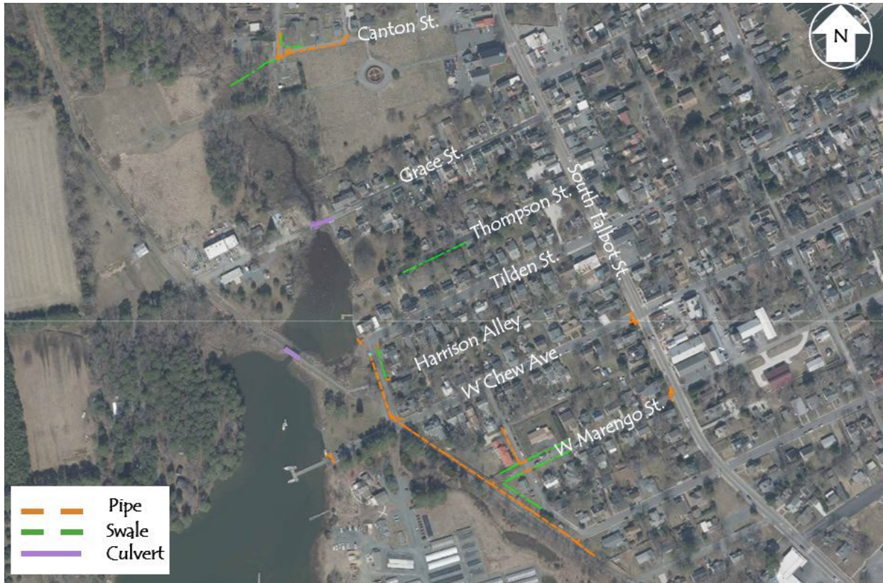
Figure 4 - Stormwater Management Features
