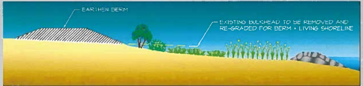
Figure 18 - Replacement of Bulkhead with Berm & Living Shoreline
